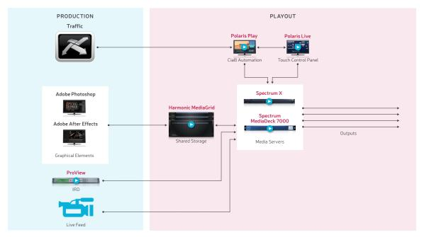
Harmonic's iMCR solution, featuring Spectrum media servers, Polaris Play automation and the Polaris Live touch control panel
