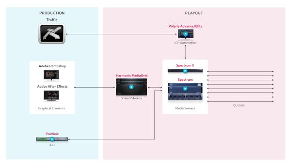
Harmonic's ICP solution, featuring Spectrum media servers and Polaris Advance or Polaris Elite automation
