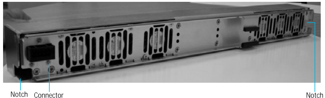
Figure 5–3: ProStream 1000 Chassis with Notches and Front Panel Connector
