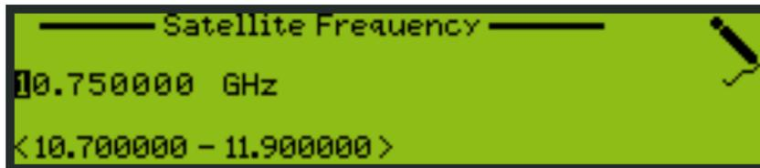
Use the <left> and <right> arrow keys to select a digit and the <up> and <down> arrow keys to change the value of the parameter. You can enter values using the alphanumeric keypad. Press <ENTER> to confirm the change or <ESC> to revert to the original value.
