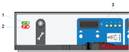
Figure 7-51: I/O module LED indicators
