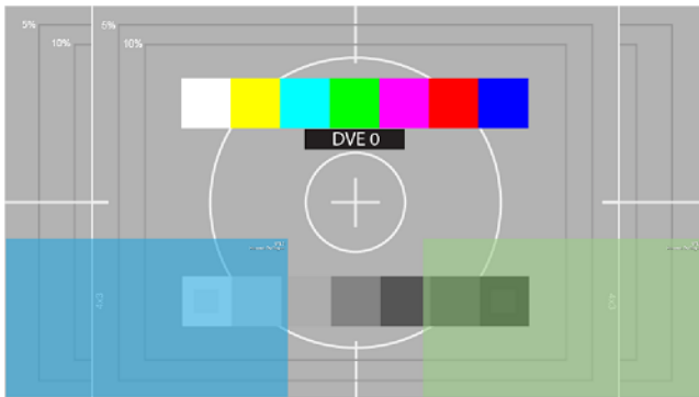
Figure 6-7: Dual DVE Dst Regions of a 4x3 Src Region, scaled and positioned in the lower corners of the screen
