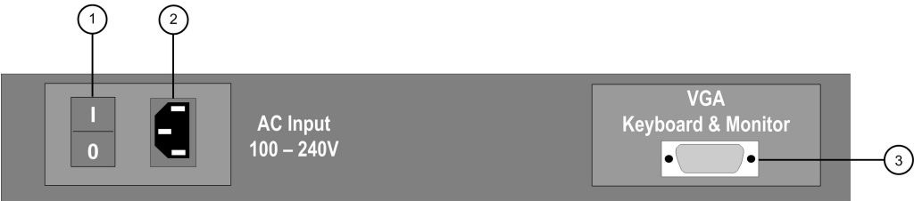
Figure 2-5: NSM-2017K keyboard/monitor unit rear panel components
