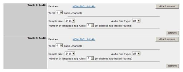
Figure 7-40: Multiple Audio Track Players Configuration Example
