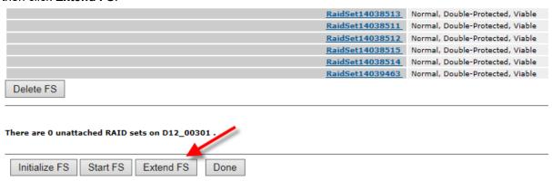
At this point, Spectrum creates new RAID sets and adds them to the file system. Depending on the size of your Spectrum system, it may take several minutes for the operation to complete and for SystemManager to display the new RAID sets in your file system.
